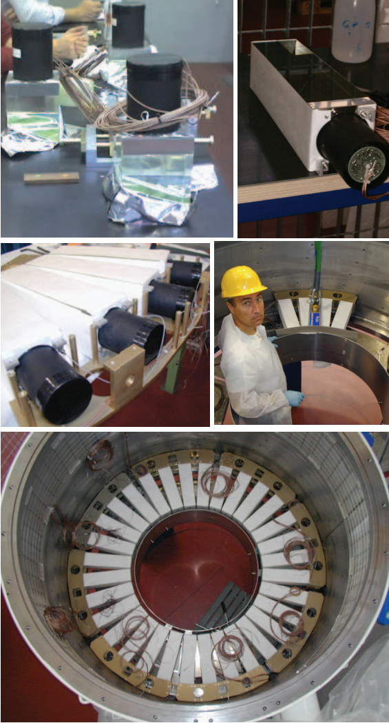
Figure 2: LAV station assembly phases (from top-left): cabling of PMT, wrapping of crystals, mounting of four-crystals brackets, fixing of brackets inside the steel cylinder, routing of cables to vacuum flange ports.
