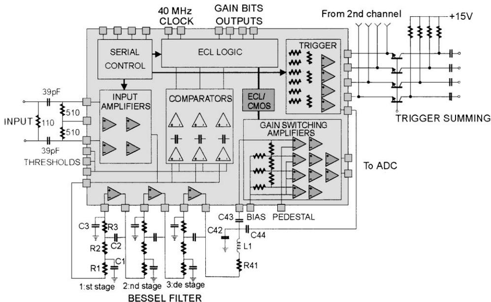
Fig. 3. Block diagram of the KRYPTON ASIC with external components.
