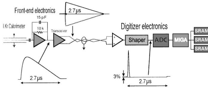
Fig. 1. Signals at various parts of the LKr electronics.
