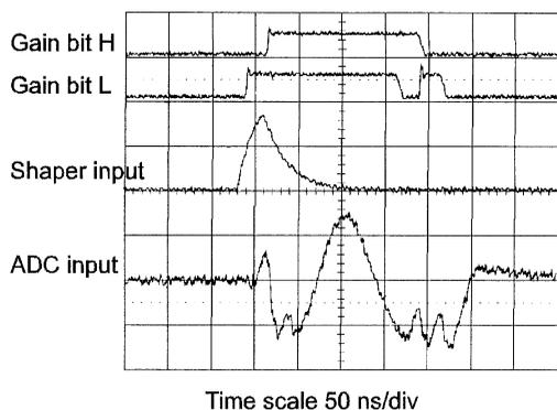
Fig. 2. Digital gain bits, signal at the Bessel filter input, and analog input at the ADC for a step input signal.
