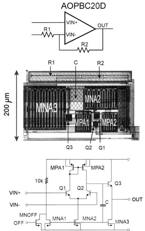
Fig. 4. Block diagram, layout and schematic of the op-amp.
