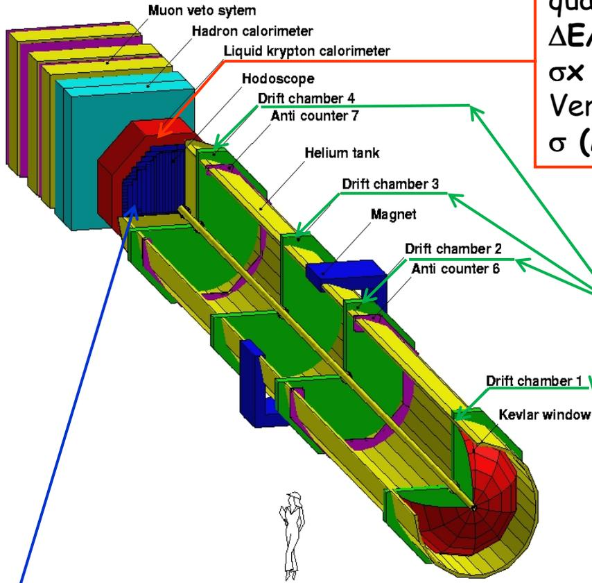
**Hodoscope for charged fast trigger**
