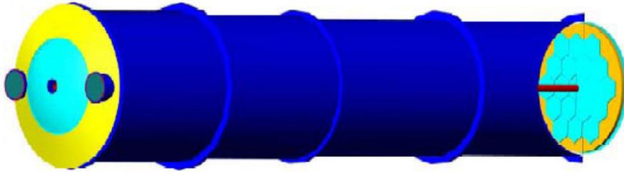
**FIGURE 1.** Schematic drawing of the RICH detector; the downstream section of the vessel is cut to show the mirrors and the beam pipe; the upstream section shows the PM assembly.
