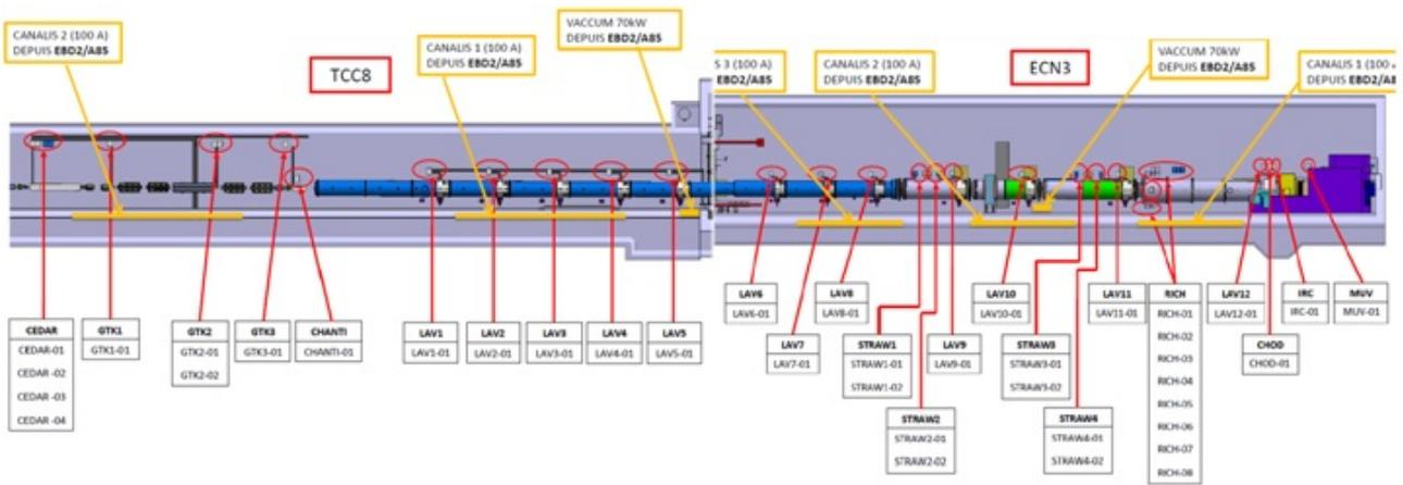
Figure 2: Layout of NA62 sub detectors.
