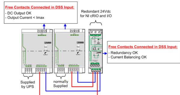
Figure 5: Redundant 24Vdc power supplies.
