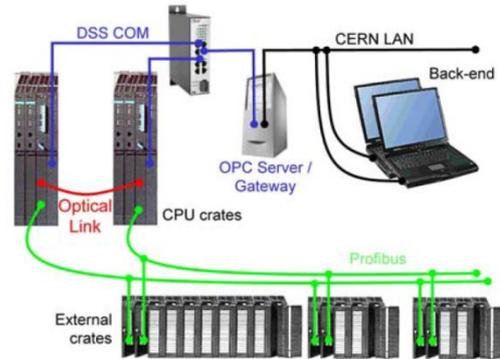
Figure 1: LHC Detector Safety System.
