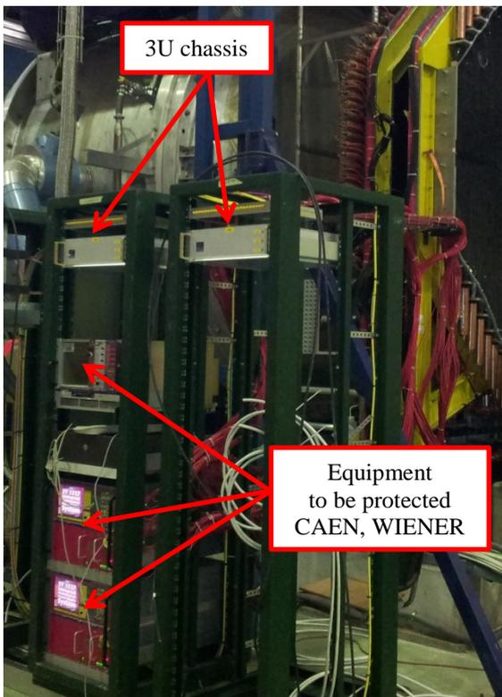
Figure 4: 3U chassis in experiment.
