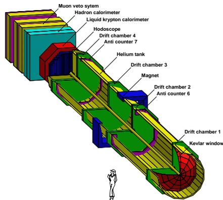
Figure 1. The NA48 detector.
