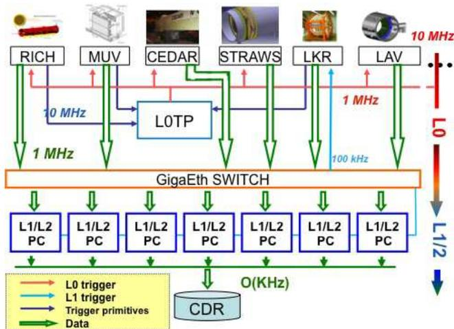
Fig. 5. TDAQ system of the NA62 experiment.
