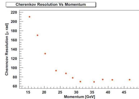
Fig. 3. Angular resolution of the RICH prototype for the 2009 beam test.
