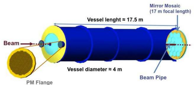
Fig. 2. RICH detector of the NA62 experiment.
