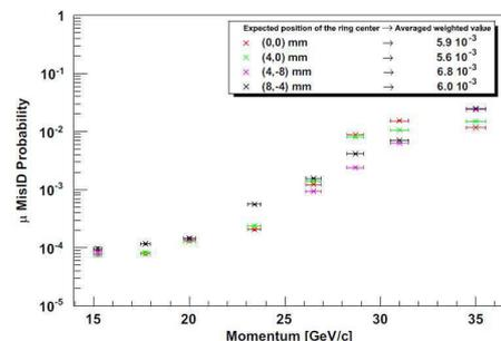
Fig. 4. Muon-pion separation for the 2009 beam test of the RICH prototype.
