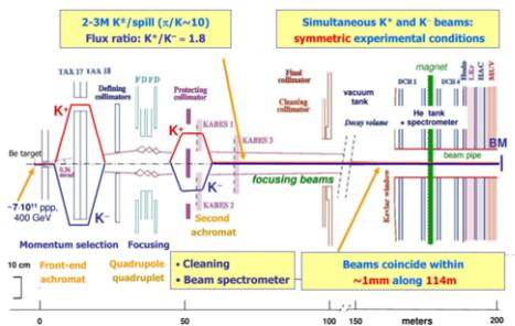
**Fig 1:** Schematics of the NA48/2 experiment using high intensity beams of charged kaons. The experiment has operated these intense beams during two runs of 50 and 60 days to measure
