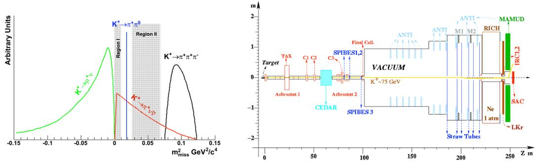
**FIGURE 7.** Experimental concepts in the P326 project: the  $m^2_{\text{miss}}$  distribution for the signal events and for the main background decays (left) and the layout of the proposed detector (right).
