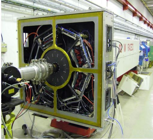
Figure 1: KTAG installed on the NA62 beamline.
