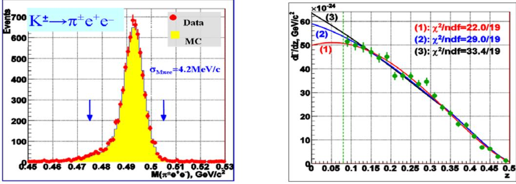
Figure 1: Reconstructed spectrum of  $\pi^\pm e^+ e^-$  invariant mass (Left) and the computed  $d\Gamma_{ee}/dz$  (background and efficiency corrected, Right) compared to fit results according to the considered models (1=linear, 2=[3], 3=[4]).
