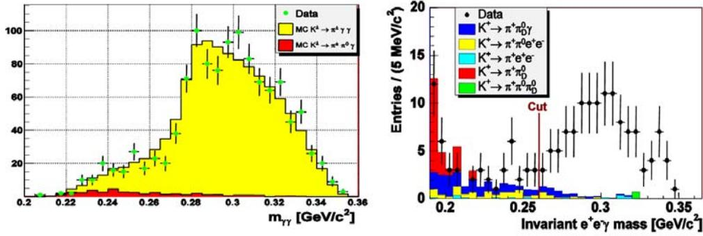
Figure 2: Reconstructed spectrum (dots) of  $\gamma\gamma$  invariant mass for  $K^\pm \rightarrow \pi^\pm \gamma\gamma$  decays (Left) and of  $\gamma e^+ e^-$  invariant mass for  $K^\pm \rightarrow \pi^\pm e^+ e^- \gamma$  decays (Right) compared to MC expectations (filled areas).
