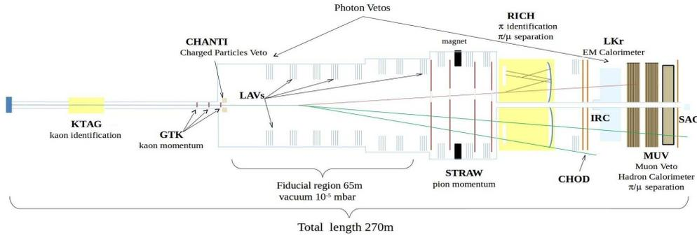
Fig. 4. – The NA62 detector layout.
