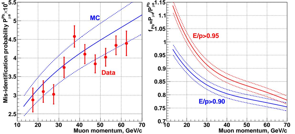
Figure 1: Left: Mis-identification probability for muons traversing the lead wall,  $P_{\mu e}^{\text{Pb}}$ , for  $(E/p)_{\text{min}} = 0.95$  as a function of momentum: measurement (solid circles with error bars) and simulation (solid line). Right: Correction factors  $f_{\text{Pb}} = P_{\mu e} / P_{\mu e}^{\text{Pb}}$  for the considered values of  $(E/p)_{\text{min}}$ , as evaluated with simulation. Dotted lines in both plots indicate the estimated systematic uncertainties of the simulation.
