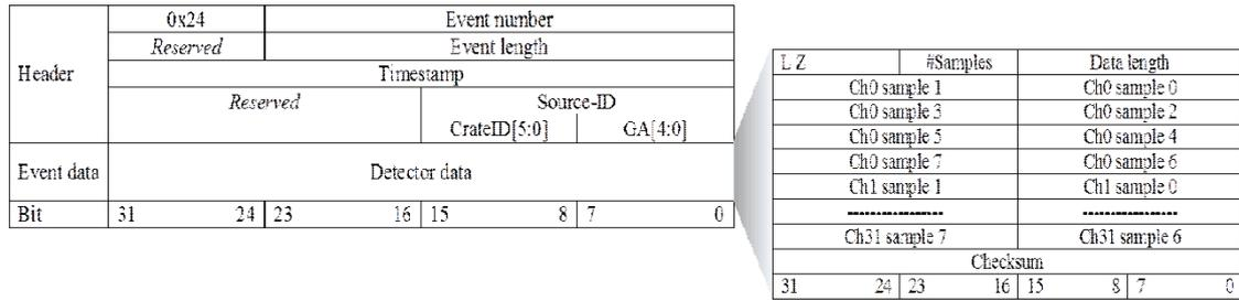
**Figure 6.** The L1 event and detector data formats.
