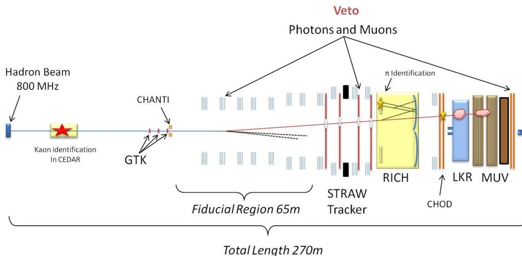
Figure 1. Schematic view of the NA62 experiment sub-detectors.
