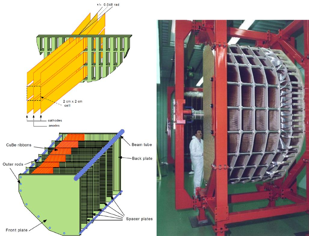
**Figure 2.** Assembled LKr calorimeter structure and electrode details.
