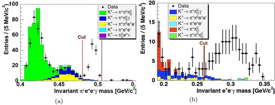
Fig. 7.  $K^\pm \rightarrow \pi^\pm e^+ e^- \gamma$  decay: selected signal candidates and background expectation from MC simulation. Vertical lines indicate the accepted region for the BR measurement. (a)  $\pi^\pm e^+ e^- \gamma$  invariant mass, (b)  $e^+ e^- \gamma$  invariant mass.
